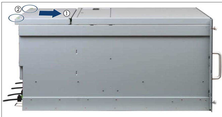
Figure 9: Installing the rear cover
